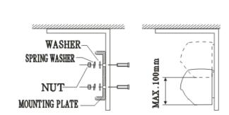
4.3.4 Hang the main body onto the upper end of the mounting plate, and then tighten the bottom fixing screws back to the mounting plate.
