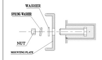
4.1.2 Determine the mounting location with the mounting plate. Secure the bolts in place. (Fill cement into the bolt holes if needed)
