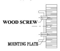
4.2.2 Hang the main body onto the upper end of the mounting plate, and then tighten the bottom fixing screws back to the mounting plate.
