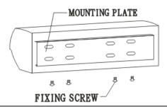
4.1.3 Tighten the nuts to secure the mounting plate to the wall after cement setting (use the washers and nuts as the Fig shows).
