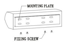
4.3.1 Remove the mounting plate from the main 4.3.2 Securely mount the ceiling brackets (not included) as the Fig shows.
