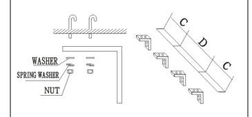
4.3.3 Fix the mounting plate to the ceiling brackets and tighten it securely as the Fig shows. The position of the mounting plate can be adjusted in vertical direction according to need, but the max distance is 100mm.
